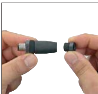
1. Unscrewing the PG7 cable gland
