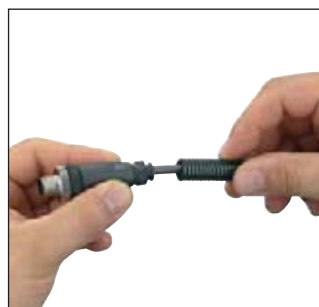
3. Fitting a PG7 protective sleeve
