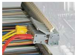
Testing with test plug modules.
