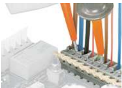
Testing with test probes.
