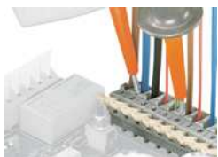
Testing with test probes.
