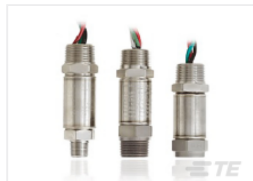
TE Part #11108663-00 300 PSI, 1/4MNPT, 4-20mA, Conduit, 18AWG
