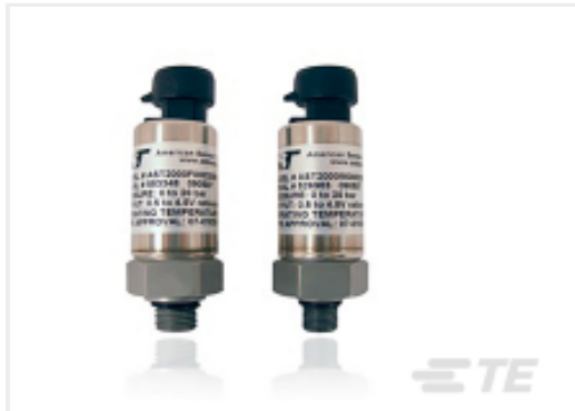
TE Part # 11104118-00 448 BAR, 7/16-20UNF Male, 0.5-4.5V ratio
