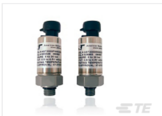
TE Part #11104118-00 448 BAR, 7/16-20UNF Male, 0.5-4.5V ratio
