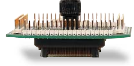
Fig. 4: Clip with internal locking feature
