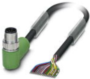
Sensor/actuator cable, 17-position, PVC, black RAL 9005, Plug angled M12 SPEEDCON, A-coded, on free cable end, cable length: 10 m
