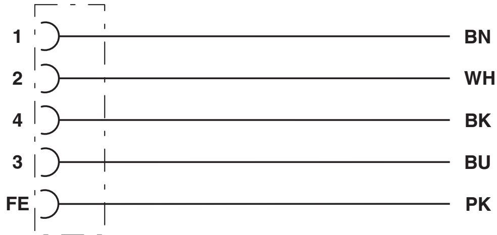
Contact assignment of the M12 socket
