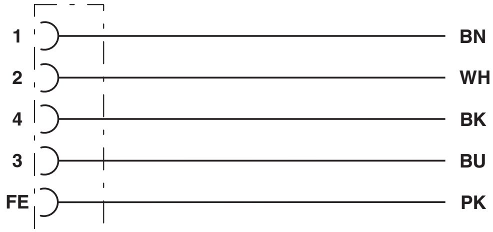
Contact assignment of the M12 socket
