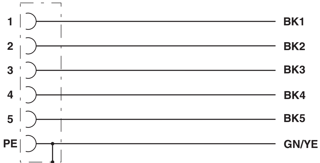
Contact assignment of the M12 socket
