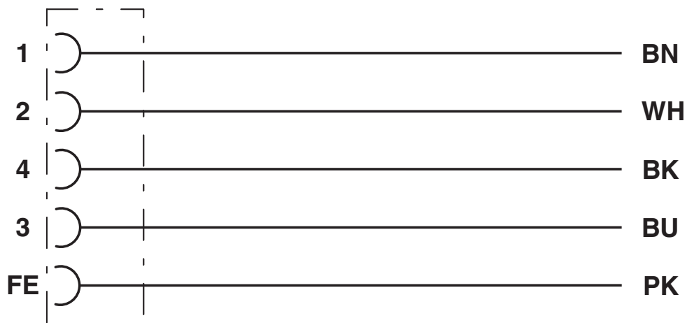
Contact assignment of the M12 socket
