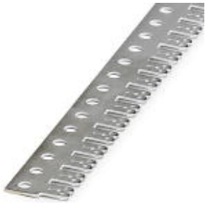
Potential busbar, with slotted 6.3/2.8 mm flat connectors, max. 40 A, brass, tin-plated, length: 1 m
