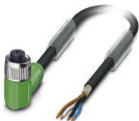
Sensor/actuator cable, 4-position, PUR/PVC, gray RAL 7001, shielded, free cable end, on Socket angled M12, A-coded, cable length: 5 m
