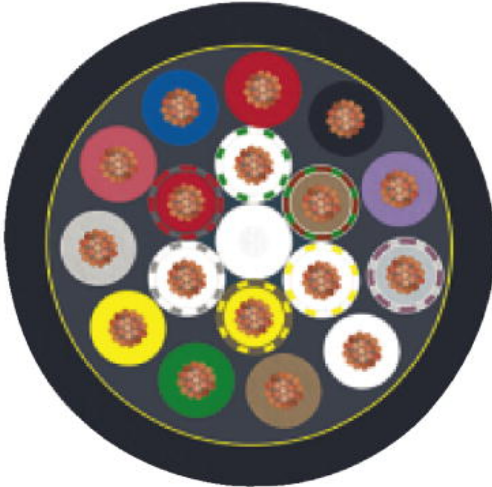
Cable cross section
