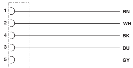
Contact assignment of the M12 sockets
