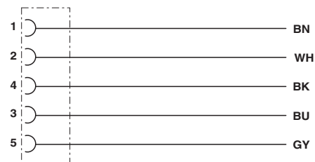
Contact assignment of the M12 sockets
