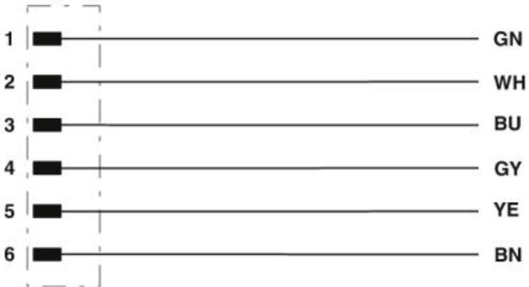
Contact assignment of the 7/8" plug
