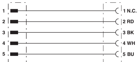
Contact assignment of 7/8" plugs/sockets
