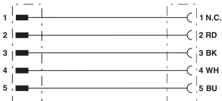
Contact assignment of 7/8" plugs/sockets
