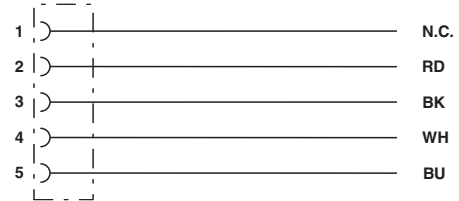
Contact assignment of 7/8" socket
