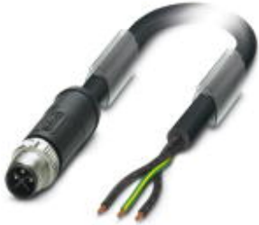
Power cable, 3-position, PVC, black, Plug straight M12, S-coded, on free cable end, cable length: 10 m, for AC current up to 16 A/230 V
