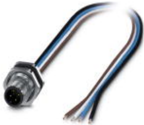
Flush-type connector, Universal, 5-position, Plug, M12, A-coded, Rear mounting, M16 x 1.5, Individual wires, cable length: 0.5 m
