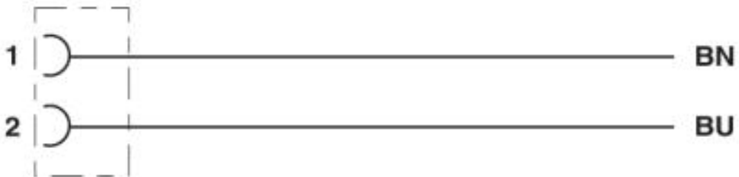
Contact assignment of the DEUTSCH DT06-2S
