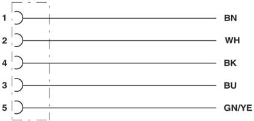
Contact assignment of the M12 sockets
