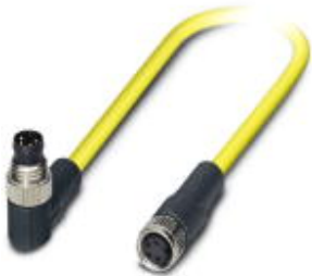
Sensor/Actuator cable, 4-position, PVC, yellow RAL 1021, Plug angled M8, on Socket straight M8, Cable length: 1.5 m
