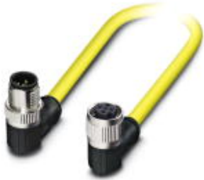
Sensor/Actuator cable, 5-position, Variable cable type, Plug angled M12 SPEEDCON, A-coded, on Socket angled M12 SPEEDCON, A-coded, Cable length: 1.5 m
