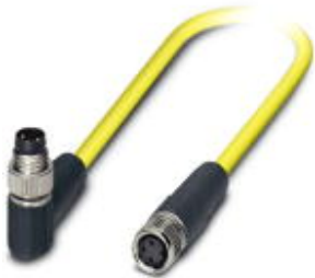
Sensor/actuator cable, 3-position, PVC, yellow, shielded, Plug angled M8, on Socket straight M8, cable length: 0.5 m
