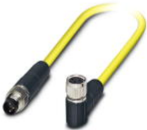
Sensor/actuator cable, 3-position, PVC, yellow, shielded, Plug straight M8, on Socket angled M8, cable length: 0.5 m
