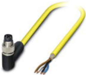
Sensor/actuator cable, 4-position, PVC, yellow, shielded, Plug angled M8, on free cable end, cable length: 10 m
