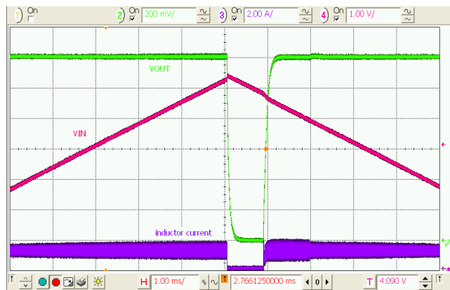
Figure 29. Input Over-Voltage Protection
