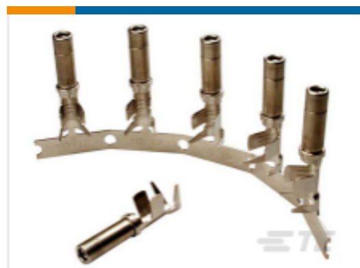
TE Part # 1062-12-0222 SOCKET, S&F, SIZE 12, 10AWG, NICKEL
