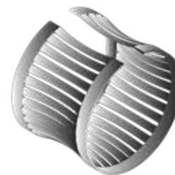
Figure 2. Conventional Contact on the left, LouverBand Contact on the right
