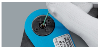
STEP 4: Insert the wire in the contact.
