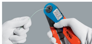
STEP 5: Tighten the crimping tool.
