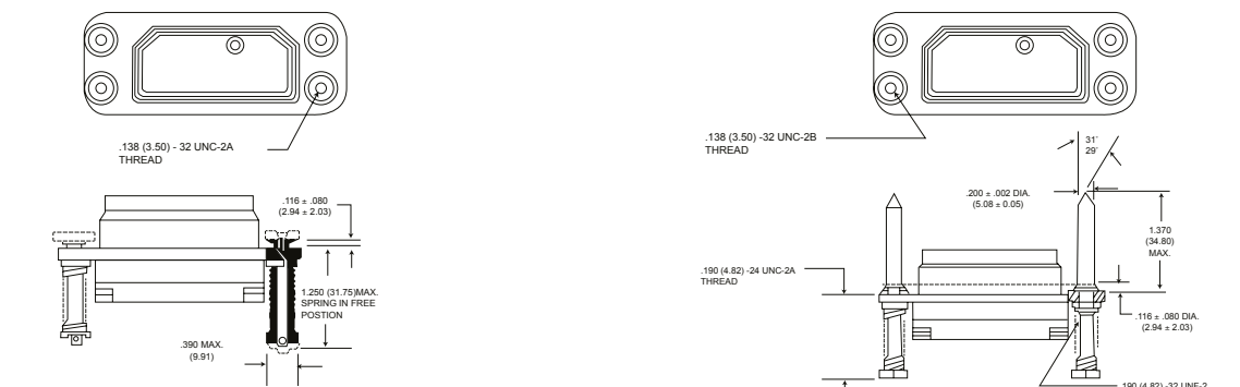
Mounting Style K With Captive Springs
