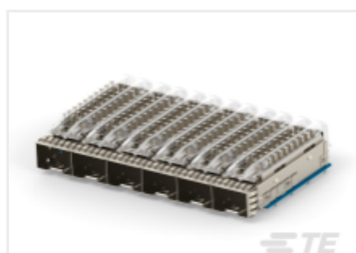
TE Part #2293156-2 ZSFP+ 1X6 CAGE ASSY, PRESS-FIT, HS
