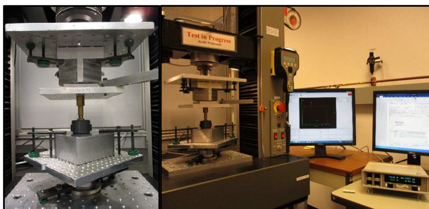
Figure 11 – Typical Receptacle Mounting Torque Test Setup
