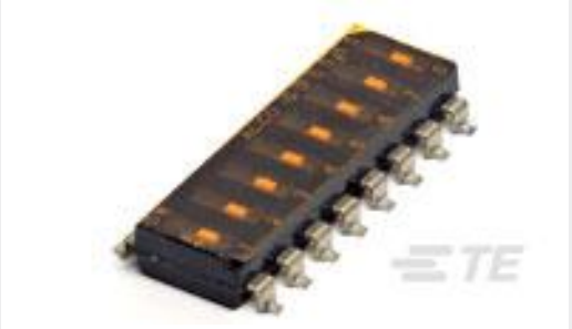
TE Part #1-1825006-9 GDS10S04=DIP SW,SLIDE,SMT
