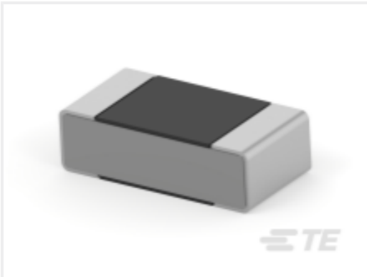
TE Part #8-1879130-1 RN 0402 4K99 0.1% 10PPM 5K RL
