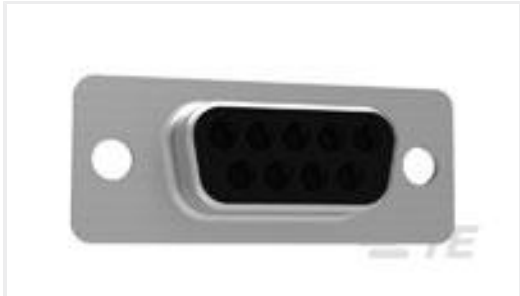
TE Part #5-747905-2 9 Rcpt Solder Cup, Gold Flash,
