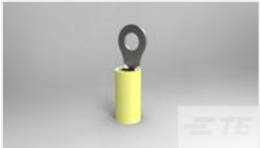
TE Part #8-324075-1 TERMINAL,PIDG R 26-22 10
