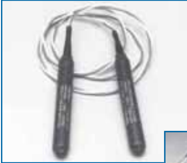
ARINC 629 Cable with Terminators
