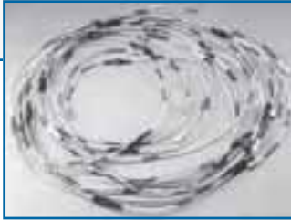
ARINC 629 Cable with Cable Couplers
