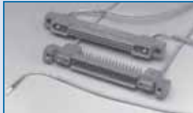
Low Mating Force PCB Connector with Combination of Signal Brush Contacts and Fiber Optic Termini
