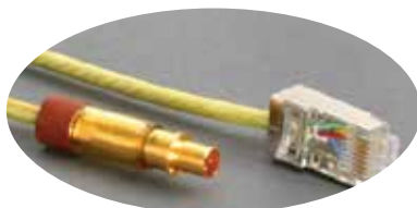
Quadrax Pin with 8P8C "RJ45" Jack
